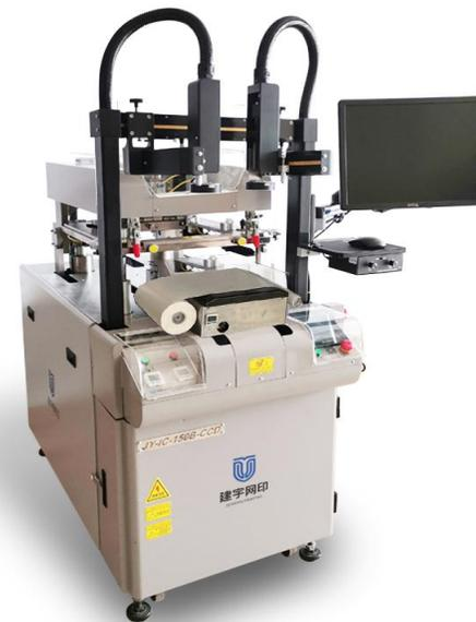
**IC-150B-LTCC厚膜印刷机**
