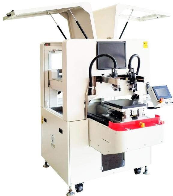
**HG-250-CCD厚膜印刷机**
